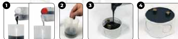
Mix the 2 components in a ratio of 1:1.
